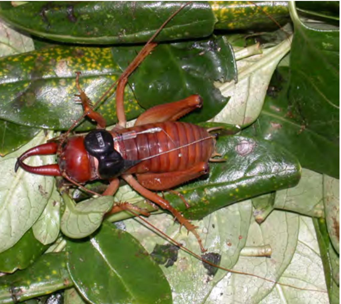
Adult male tusked wētā with micro-transmitter. The harmonic radar transponder is visible beneath the transmitter with the diode projecting back on the right. The transponder aerial is the fine wire from the diode that is bent to the left and passes under both the transmitter aerial and the left femur. Photo: Danny Thornburrow
